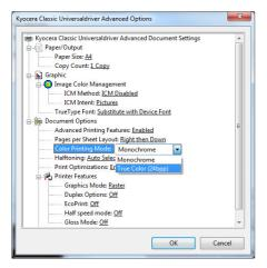
Move to 'Color Printing Mode:' (Farbdruckmodus:) and switch the setting to 'True Color (24bpp)'.
