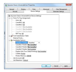
'Paper Feeder:' and 'Duplex Unit (..):' should be set-up at installation time (Vista and newer). If not please make the correct settings here.
